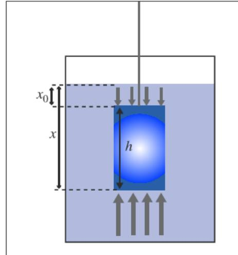
Fig. 1(b). Schematic representation of the pressure forces acting on top and bottom surfaces of a body totally immersed in a liquid.
